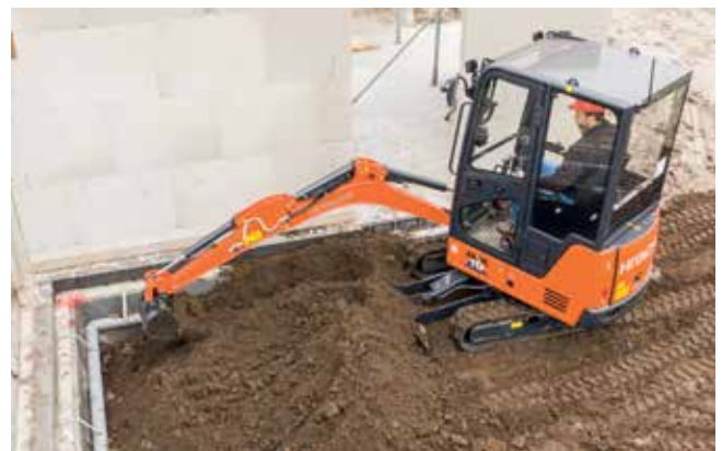
Small front minimum turning radius is ideal for narrow spaces.
