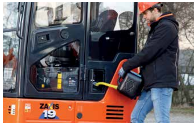
Relocated fuel tank opening allows for easy refuelling.
