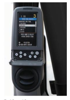
**Tool Control System.** The optional tool control system maximizes work tool productivity by configuring hydraulic flow, pressure, and operator controls to match a specific work tool. System versatility enables a wide range of tools to be used.
