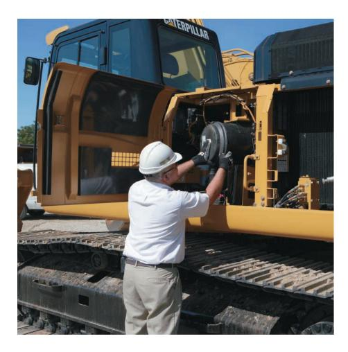
**Ground Level Service.** The design and layout of the 336D was made with the service technician in mind. Many service locations are easily accessible at ground level allowing critical maintenance to get done quickly and efficiently.
