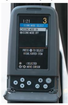
**Monitor.** The monitor is a full color 400x234 pixels Liquid Crystal Display (LCD) graphic display. The monitor angle can be adjusted to minimize sun glare and has the capability of displaying information in twenty-seven different languages.
