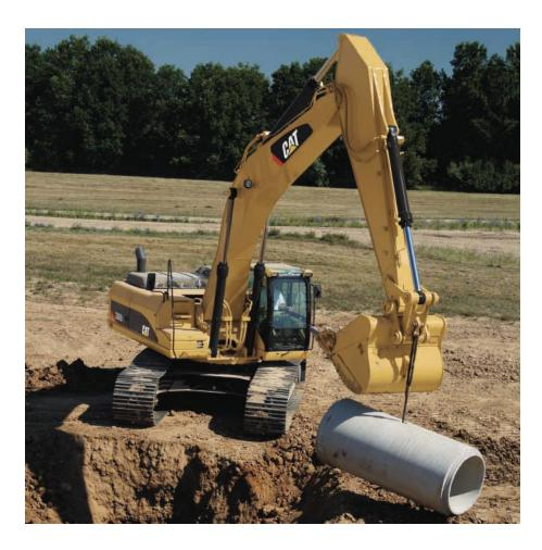
Auxiliary Hydraulic Valve. The auxiliary valve is standard on the 336D. Control Circuits are available as attachments, allowing for operation of high and medium pressure tools such as shears, grapples, hammers, pulverizers, multi-processors and vibratory plate compactors.
